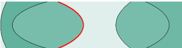
Figure 26. Cross section of two lens pairs with the default color table “White and Mint”. Air is marked light green. Glasses are marked by different shades of dark green. The third surface is currently selected and thus marked red.
