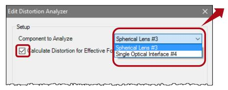
Select a lens component to be analyzed. The analysis is independent of the system.
