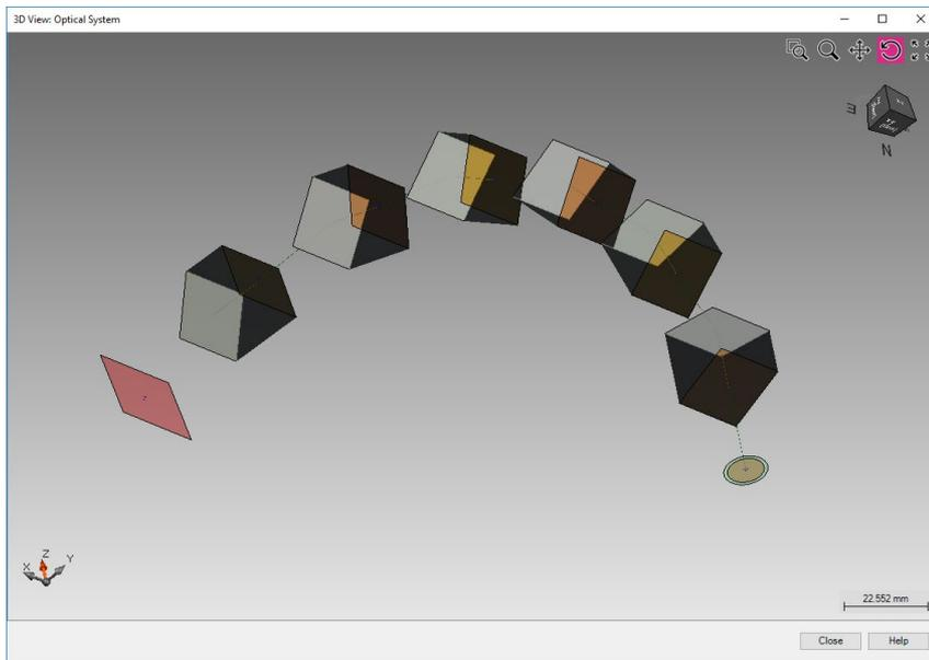
Computer Aided Design files are often used to exchange files between software products. STL format for example is used in 3D printing software. IGES format is widely used for the digital exchange of information in the field of Computer-Aided Design (CAD). VirtualLab Fusion supports the export of optical components specified in the system into various CAD formats. This includes for example the export of lenses, prisms, mirror systems and other components into STL and in IGES format.
